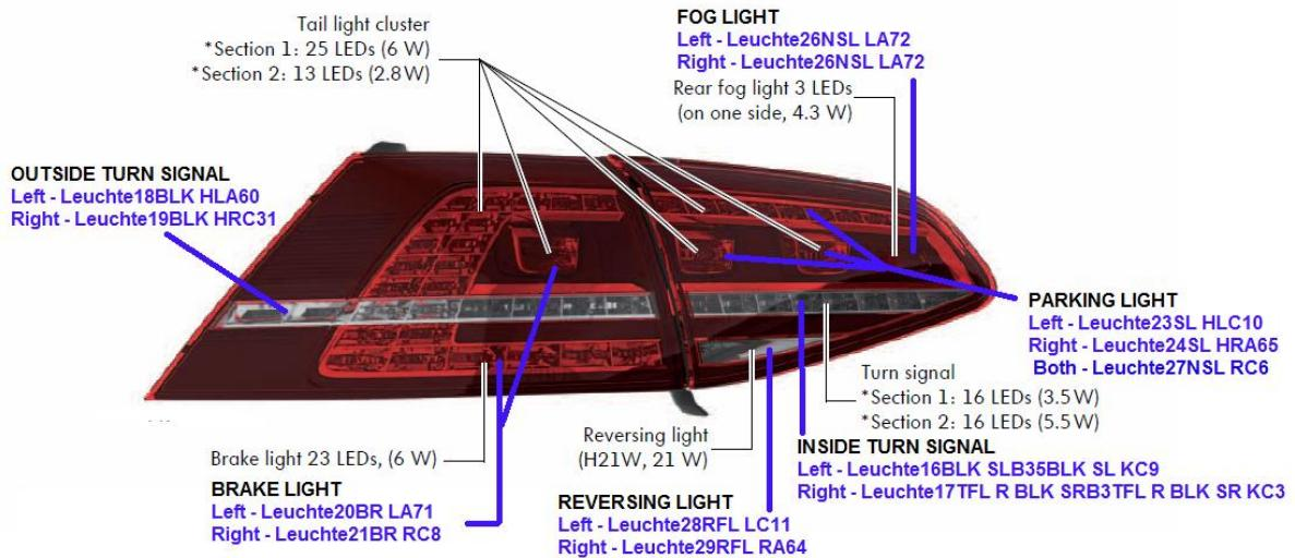
\*Section 1 = outer tail light cluster; \*\*Section 2 = tail light cluster in the tailgate
